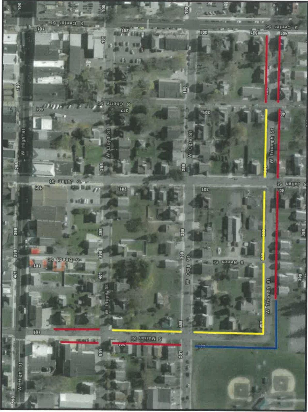
South Marian Street & West Triumph Street Red = Curb & Sidewalk Yellow = Curb Only Blue = Sidewalk Only
