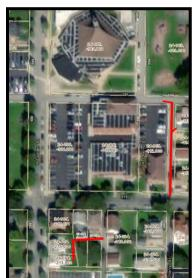
sewer main existed between the private sewage collection network and Truman Street and had significant I&I. Guyer offered to replace that section of public main at a cost of \$11,000. That additional work was approved. Such a price (\$45/LF plus restoration) could not have been obtained through bidding and was below the bidding threshold.
